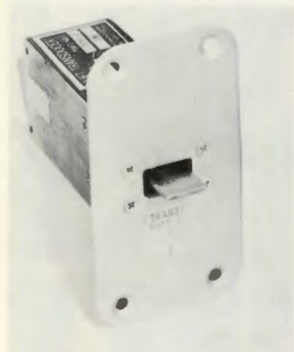
Probe from the Beech. Whole unit is heated to preclude icing.
